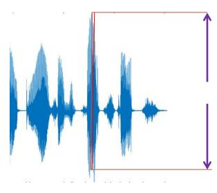
V = largest volts swing at any instant. Scope best method. Normally one or two cycles only. With scope, apply cursors to show the narrow peak and read voltage in this area. This is PTP voltage. ½ is Peak voltage
