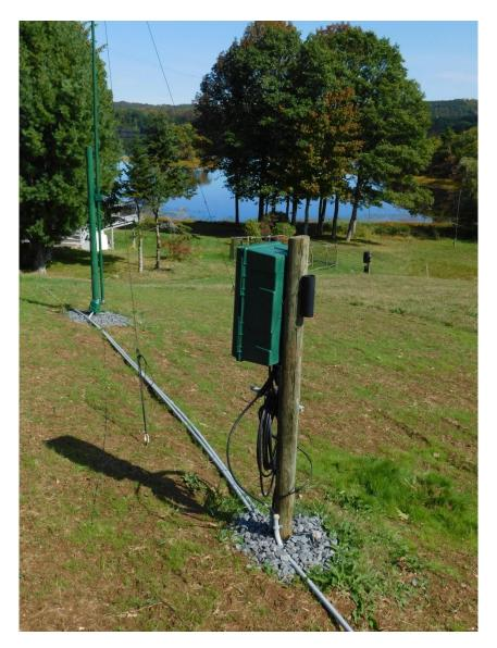
In this picture you can just see parts of the dual delta loop array located down the slope from this vertical array. Down by the lake shore is a SAL20 receive array. The small plastic tube on the back of the mounting post holds a golf umbrella to provide shelter on sunny or wet days while working in the control box.
