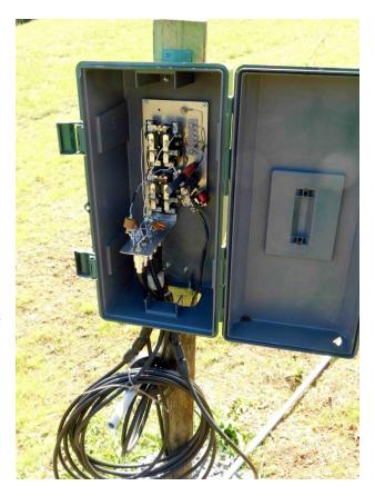
The <u>measured</u> feed point impedance after building was 37 -j20.3 in one direction, and 40.2 -j16.7 in the other. Not bad. To lower the reactance slightly would only require a capacitor, in addition to the feedline capacitor to isolate the DC control signal from the RF.
