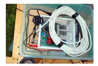
The inside of the base container showing the stub, the choke and the MFJ927 that destroyed itself last year. It's now replaced by an SGC239 Smart tuner, with the addition of a bias T and some RF connectors. (Note, there is a detailed explanation of this antenna, plus problems encountered with the first MFJ auto tuner on my VE1ZAC website)
