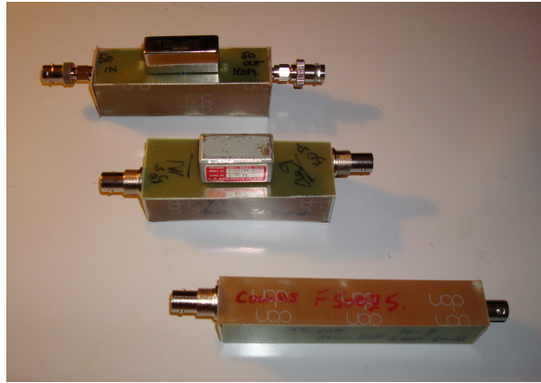
Figure 2: Typical filters, mounted in RF tight housings with internal matching networks or transformers
