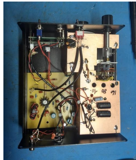
Figure 10 Oscillator shield , power supply and 160 filter
