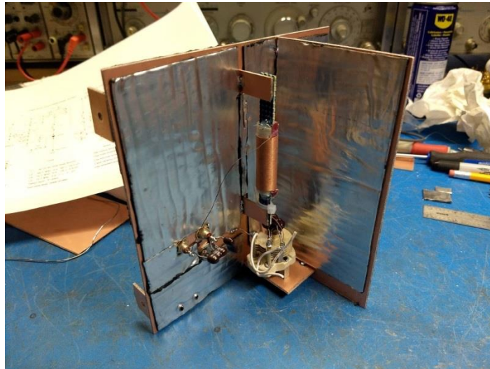
Figure 3 Internal dividers and oscillator coil/cap compartment
